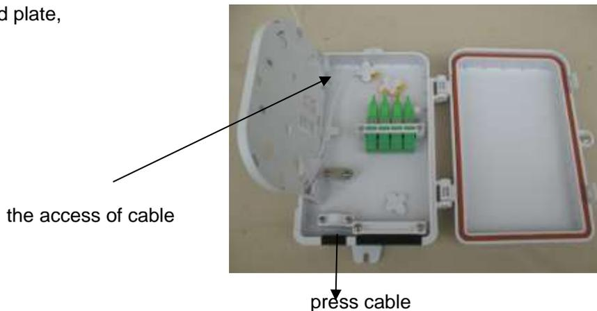
2, Introduce the cable from the bottom of the splice tray to joint with the pigtails, then splice them, please twist the rest of the pigtails well with the cable. Splice as usual, then put the splice protective tube into the slot of tray.
