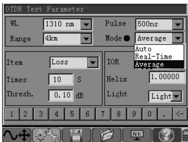
Fig.2-10 Setting of test modes of 5302 OTDR
