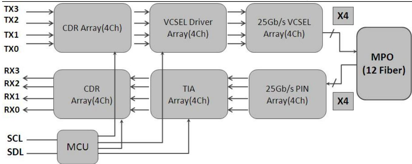
\* 100GBASE-SR4 QSFP28 is one kind of parallel transceiver. VCSEL and PIN array package is key technique, through I2C system can contact with module.
