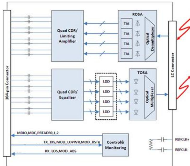
**Figure 1. CFP4 LR4 Optical Transceiver functional block diagram**
